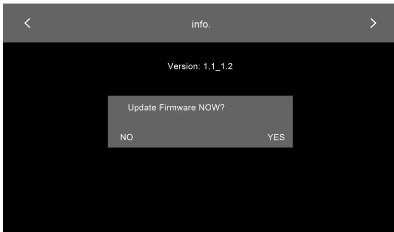
3.) The system will auto shut down when the upgrade is done. The LED of the probe tip will keep flashing while the update is ongoing
