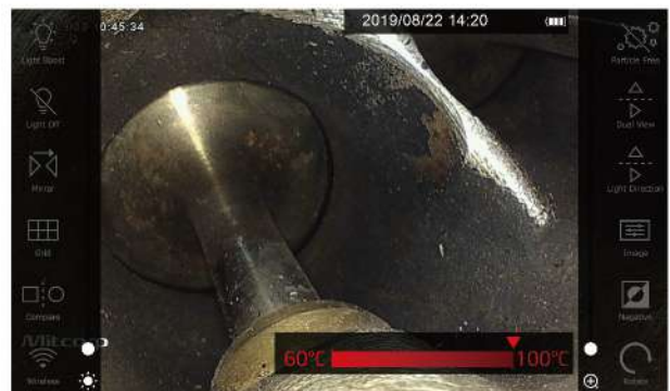
3 stage temperature warning & auto shut down function
