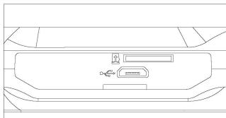
The device is equipped with a TF memory card(inserted). Gently press to eject the card.
