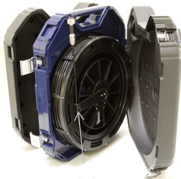
Fig. 72: Rod guide in the end position
