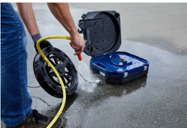
Fig. 69: Cleaning the viper and the rod
