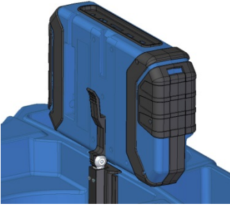
Fig. 63: Press lever and pull the monitor from the support at the same time.
