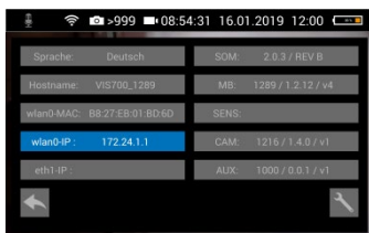
Fig. 55: Info-menu with the WLAN-Access-Point-mode activated.
