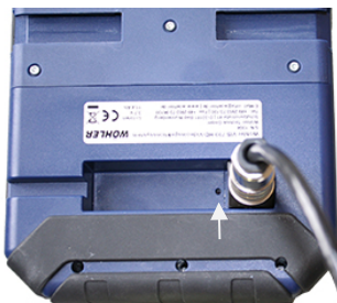
Fig. 61: Reset hole indicated by an arrow
