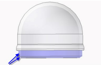
Fig. 62: Fitting the camera dome
